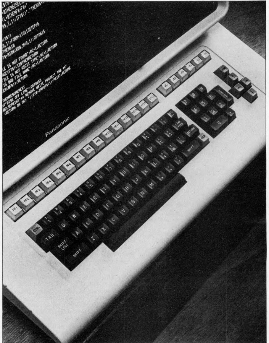
A close look at the Panasonic's comprehensive keyboard. Opposite: when scrolling, the characteristic high screen persistence causes severe "ghosting" of the image.
